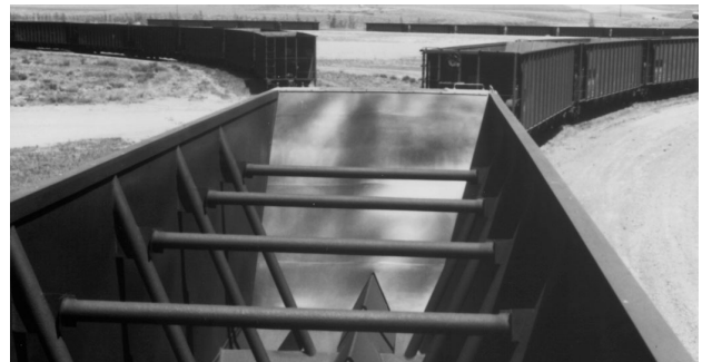
Basin Electric railcars with TIVAR® 88-2 liners installed.
